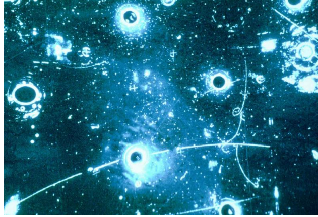
Figure 44. The first detection of neutral currents. The neutrino came in somewhere at the top and sent an electron barreling downwards, creating a shower of e^+e^- pairs, with their tell-tale spiral tracks. A black and white version of this appears in the discovery paper “ Search for Elastic Muon-Neutrino Electron Scattering ”. The same journal contains a second paper with evidence for neutral currents from hadrons.
